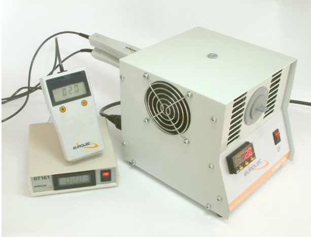
CS174 with RT162 & PC Temp PT2 portable thermometers CS Series Dimensions (l x w x h) 196 x 174 x 179mm
