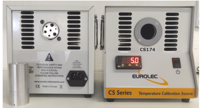
CS174-IN version rear view showing removable insert CS174 front view with black body cover removed
