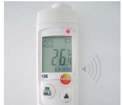
Audible and optical alarm (LED lights up)
